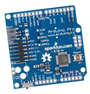
over-current protection and a maximum output of 150mA. The Arduino Pro board does not have connectors populated so that any connector or wire can be soldered with any orientation.
