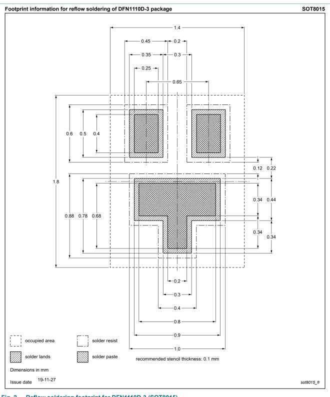
Fig. 2. Reflow soldering footprint for DFN1110D-3 (SOT8015)
