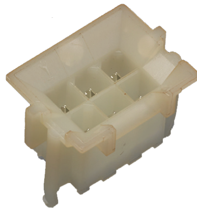
DAMAGED IN REFLOW PROCESS
