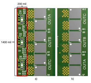
Figure 4. Example gate drive layouts for a threephase driver.
