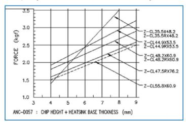
Figure 4. Typical Loads for Z-clips [3].
