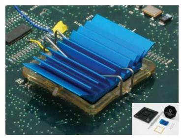
Figure 5- maxiGRIP™ Heat Sink Attachment Solution.
