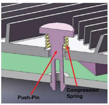
Figure 6. Cross Section View of Push-Pin & Compression Spring Attachment.
