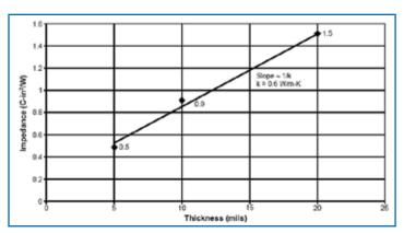
Figure 2. Graph of Tape Thermal Impedance with Respect to Tape Thickness.
