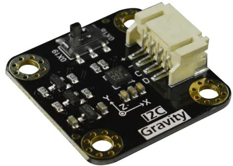
This sensor comes in user-selectable scales of  $\pm 6g/\pm 12g/\pm 24g$  and is capable of measuring accelerations with 0.5Hz to 1KHz output data rates range. This sensor operates at a 3.3V to 5V voltage range and a -40°C to 85°C temperature range. The applications are in navigation, smart agriculture, robotics, and VR/AR.
