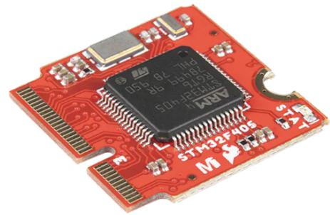
This MicroMod STM32 processor board features a Floating-Point Unit (FPU) single precision, supporting all ARM single-precision data-processing instructions and data types. The processor board implements a complete set of DSP instructions and a Memory Protection Unit (MPU), enhancing application security. This processor board utilizes the DFU bootloader to upload code and incorporates an extensive range of enhanced I/Os and peripherals.
