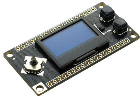
The OLED screen consists of a protective frame to protect the screen as well as the finger from getting scratched on the edge of the glass. The OLED display module integrates OLED 12864 with the GT30L24A3W multi-language font library chip and the BMA220 three-axis accelerometer. The FireBeetle covers-OLED 12864 display also features an analog directional key and two independent digital keys A and B.
