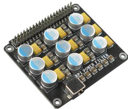
The filter board can be directly plugged into the module to the Raspberry Pi GPIO port for use. When used with an audio decoder board, the filter board turns Raspberry Pi into a high-quality stereo. Typical applications of power filter board for Raspberry Pi 3B+/ 4B include Raspberry Pi audio output.
