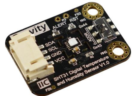
The SHT31-F sensor provides humidity accuracy of  $\pm 2\%$ RH at 0%RH to 100%RH (at 25°C) and typical temperature accuracy of  $\pm 0.2^\circ\text{C}$  at 0°C to 90°C. The SHT31-F sensor features IP67 rating that protects the sensor opening from liquids and dust. This sensor is ideal for use in urban environment monitoring, intelligent buildings, industrial automation, smart home, and other Internet of Things (IoT) applications.
