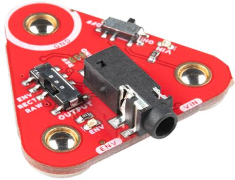
The board also includes two switches: one is used for power while the other is selecting the output mode for the raw EMG (RAW), rectified (RECT), or envelope (ENV) signal. This board comes with two status LEDs built in for power and the envelope signal.
