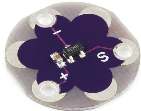
Each LilyPad is creatively designed to have large connecting pads to allow them to be sewn into clothing. There are various input, output, power, and sensor boards are available. It is also washable.
