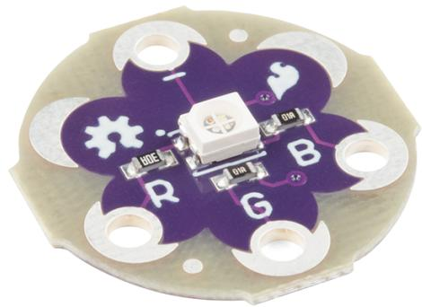
Each of the colors in the RGB LED is connected to one of the sew tabs on the board labeled R, G, and B. To light up each color individual LED, connect each LED to the power source. For simple circuit hookups, connect the R, G, and B sew tabs to power (+) and in code set them to HIGH (for digital output) or 255 (for analog output) to turn them on.
