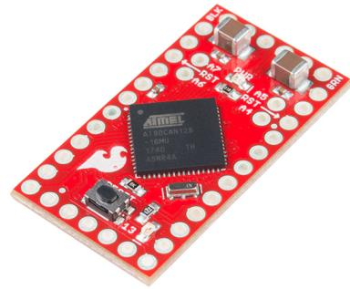
The AST-CAN485 development board features an onboard regulator which allows an unregulated input voltage to be supplied on the V<sub>IN</sub> pin to make the allowable 7V to 16V input voltage range. This board also features a 16MHz clock, 2 UARTs, 16 digital I/Os, and D13 LEDs. The AST-CAN485 development board is used in automation, industrial systems, building management, automotive systems, and OBDII applications.
