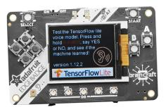
The Adafruit Arduino library features some demos for the user to get started with and to recognize various word pairs like yes/ no, up/down, and cat/dog. The user can code the EdgeBadge
