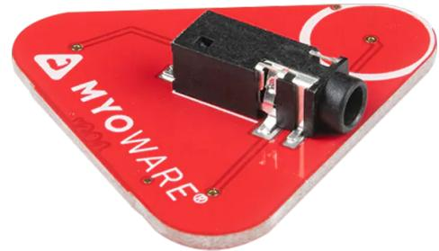
The MyoWare 2.0 Cable Shield is also equipped with snap connectors on the board so the user can easily stack it. Unlike the other shields in the MyoWare 2.0 ecosystem, this board snaps to the bottom side of the MyoWare 2.0 Muscle Sensor. Use this shield for non-wearable projects that are housed in an enclosure or that target muscles that are too small or situated such that the on-board electrode sockets would not be suitable.
