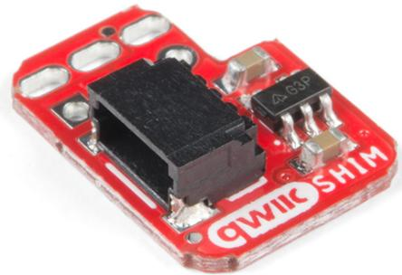
The Qwiic SHIM has a single Qwiic connector that connects to your Pi's I<sup>2</sup>C bus (SDA, SCL, 5V, and Ground). The SHIM also has a 3.3V regulator so it will work with all Qwiic devices. Even better, the SparkFun Qwiic SHIM will also work with the NVIDIA Jetson Nano Developer Kit!
