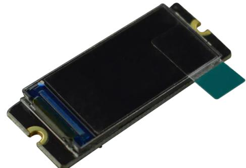
The DFR0847 display is compatible with 3.3V to 5V operating voltage range and has a current consumption of less than 15mA in full-screen. This TFT display works well with controllers like Arduino UNO, Leonardo, ESP32, ESP8266, FireBeetle M0, etc.
