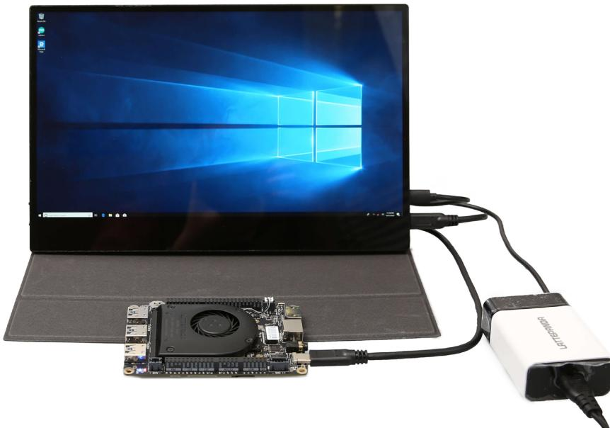
It is recommended to use the LattePanda original power adapter for power supply. The white adapter that comes with the display cannot supply power for both the display and LattePanda.
