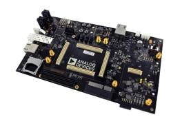
In addition, the ADRV1CRR-FMC includes an HDMI output port and several peripheral module connectors. The four serial transceivers on the SDR 1x1 and SDR 2x2 SOMs are allocated to a x1 PCIe Gen2 card edge interface, the FMC connector, a SFP+ cage, and a general purpose SMA interface.
