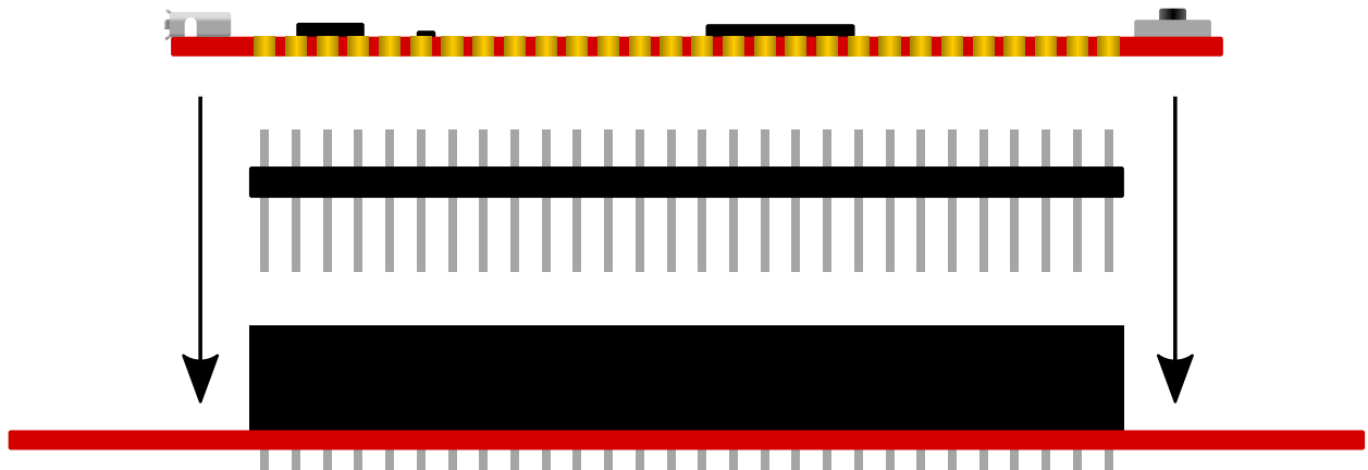
Figure 4-3. Connecting to Curiosity Nano Base for Click boards™
