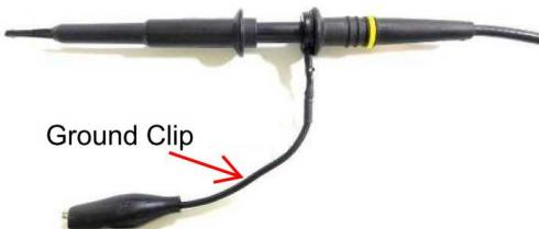
Another method is shown below, in case of coaxial-cable/BNC is not available. The noise pickup is eliminated by pressing scope probe ground ring directly against the -Vout terminal while the tip contacts the +Vout terminal. This makes the shortest possible connection across the output terminals.
