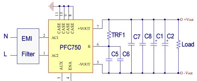
This function provides energy that maintains the output for 8ms hold up time. The capacitance in the application is recommended as follow (Allowable capacitance range: 660~2200uF).
