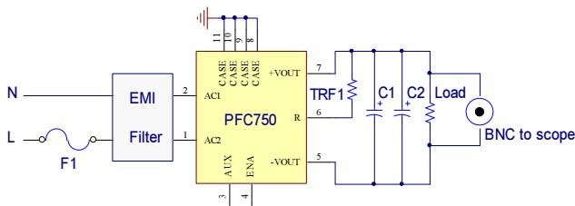
Output ripple and noise are measured with a 10uF E.L and 0.1uF ceramic capacitors across output at 20 MHz bandwidth.
