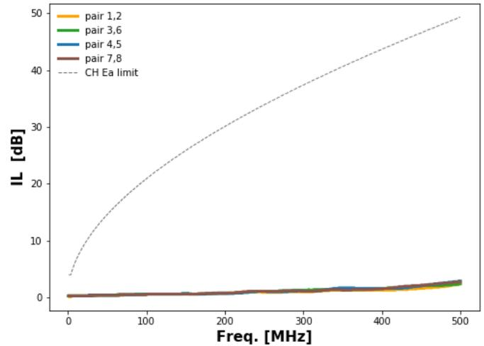
Figure 10 Insertion Loss of an EN-66 with the Class E<sub>A</sub> Channel-Link Limit
