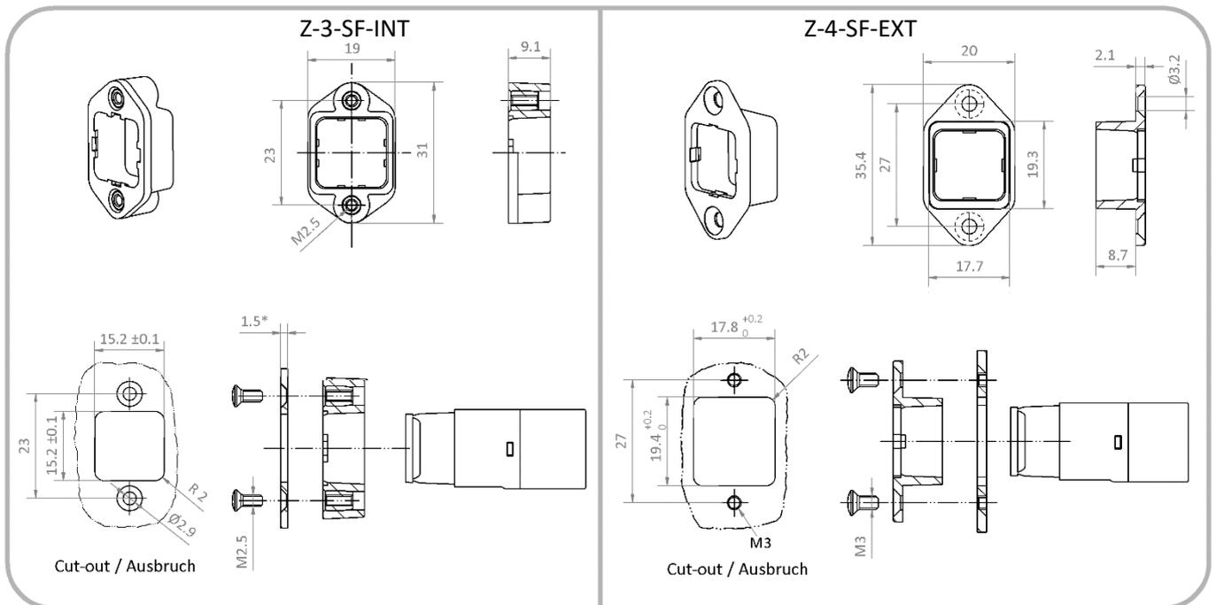
Figure 2 Physical dimensions and required cut-out for SnapFit installation frames. All dimensions are in millimetres.
