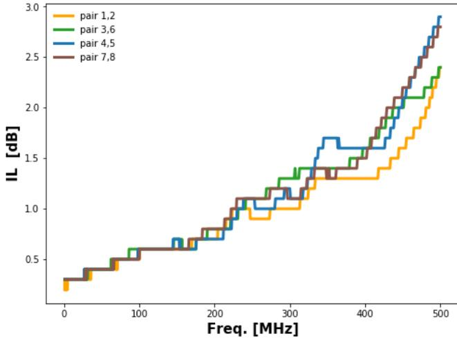
Figure 9 Insertion Loss of an EN-66
