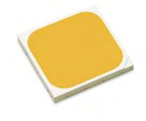
LUXEON 7070 is a multi-die, high power package that provides high luminance from a super robust package to enable cost effective, single optic and directional fixture designs. LUXEON 7070 uses an industry standard 7070 surface mount package with a small Light Emitting Surface (LES). LUXEON 7070 is offered in 70, 80, 90 CRI with a wide range of CCTs, and offers hot-color targeting to ensure that the LEDs are within color target at application conditions of 85°C.
