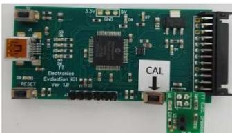
**Step 1** - Connect mainboard with daughter board containing OPB9000 samples as shown above. Daughter board orients outwards from Main board.
