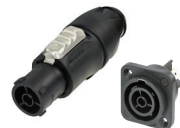
powerCON® TRUE1® TOP (3 contacts, 20A @ 250VAC) Mateable under load
