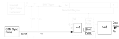
State3: Event triggered (e.g. angle synchronous) sync pulses
