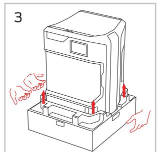
With two people lift from the side handles of the printer and put it on a stable flat surface.
