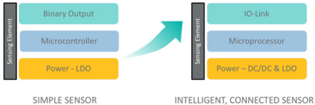
Figure 3. Intelligent, connected sensors need complex building blocks.
