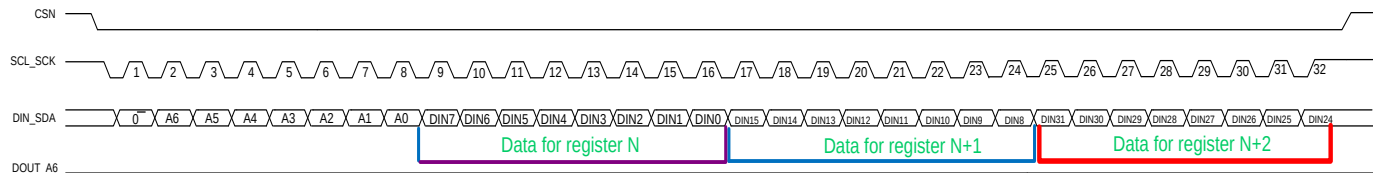
Figure 16. SPI Register Write Cycle - Burst (3-register burst example)
