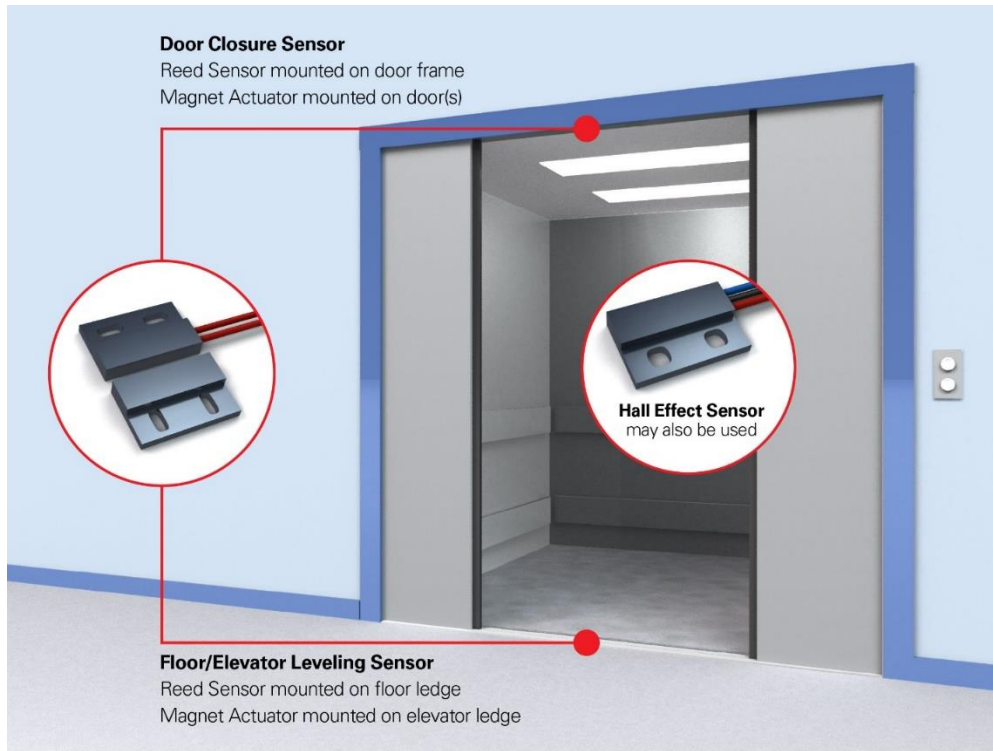
Figure 2: Reed sensors used in an elevator door
