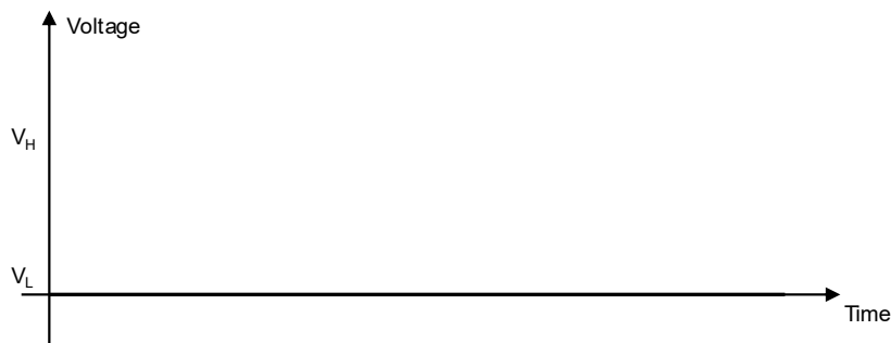
Figure 1: GPIO pin progress for no service
