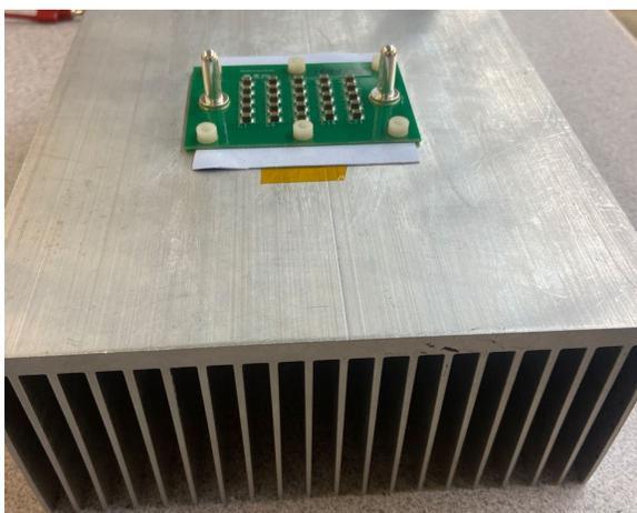
Figure 17 – 5x5 Array with large heat sink (HS1)
