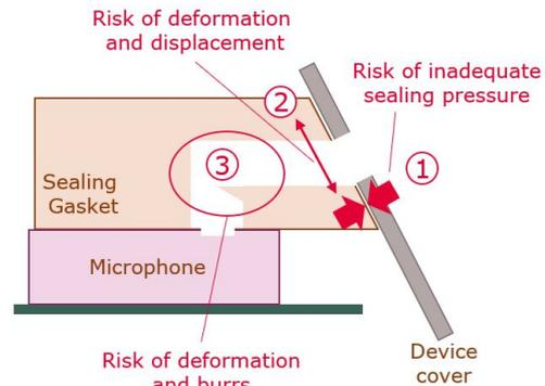
**Figure 10 Vertical surface sealing alignment**
