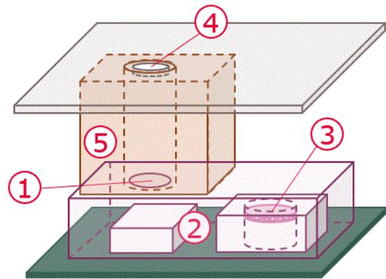
**Figure 1 Microphone acoustic channel design**
