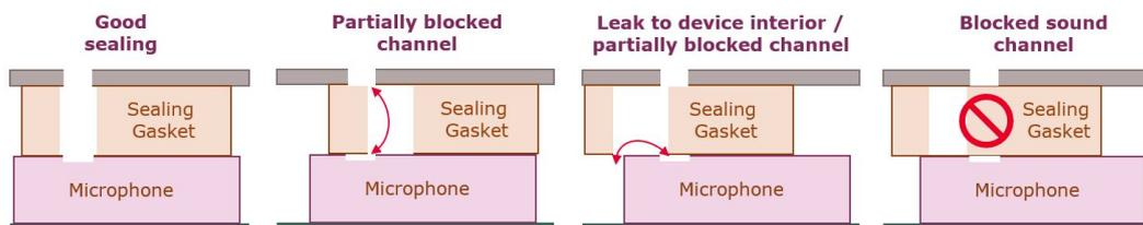
**Figure 9 Sealing alignment**
