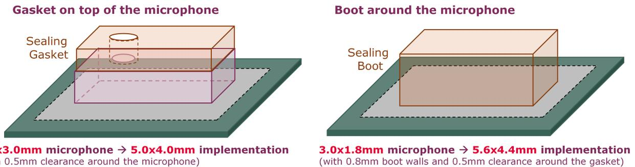
**Figure 6 MEMS microphone mechanical size implementation**
