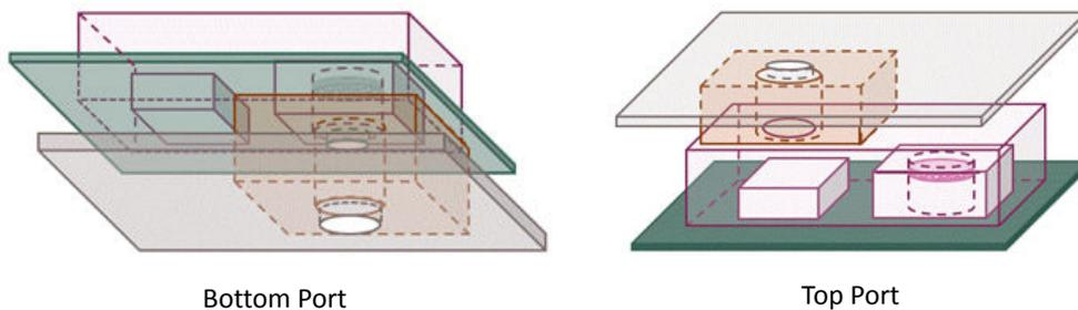
**Figure 7 MEMS microphone acoustic sealing implementation**
