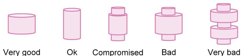
**Figure 2 Sound channel shapes**
