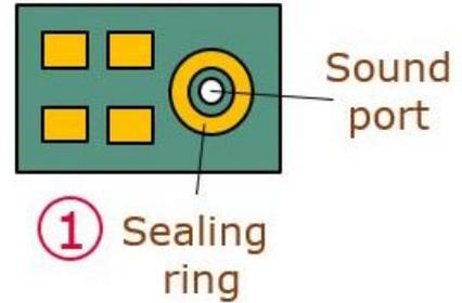
**Figure 3 Bottom view - bottom port microphone**
