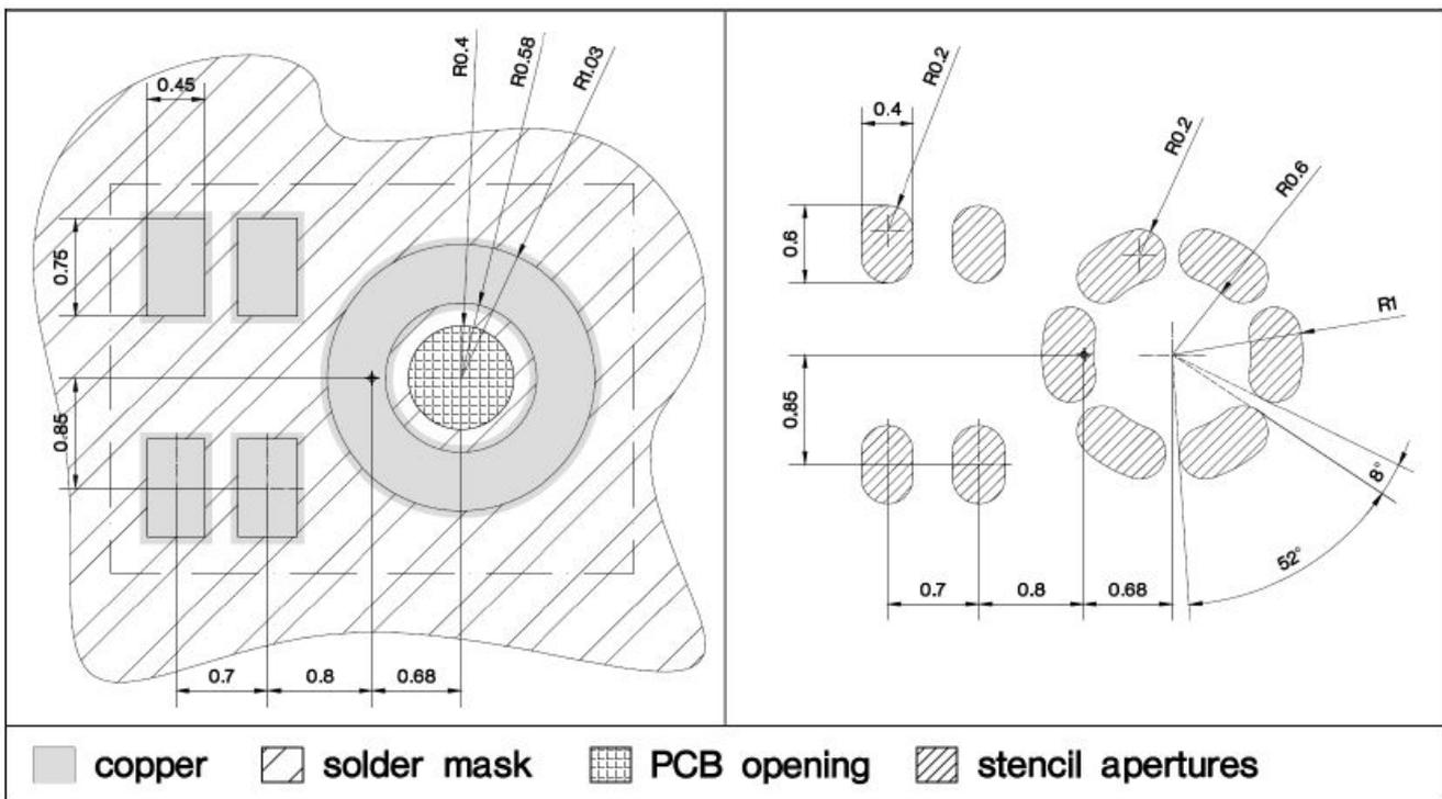
Figure 14 Infineon IM69D130 microphone footprint and stencil recommendation example
