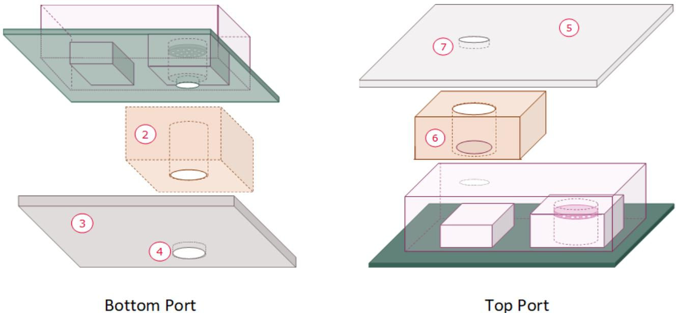
**Figure 4 MEMS microphone package type**
