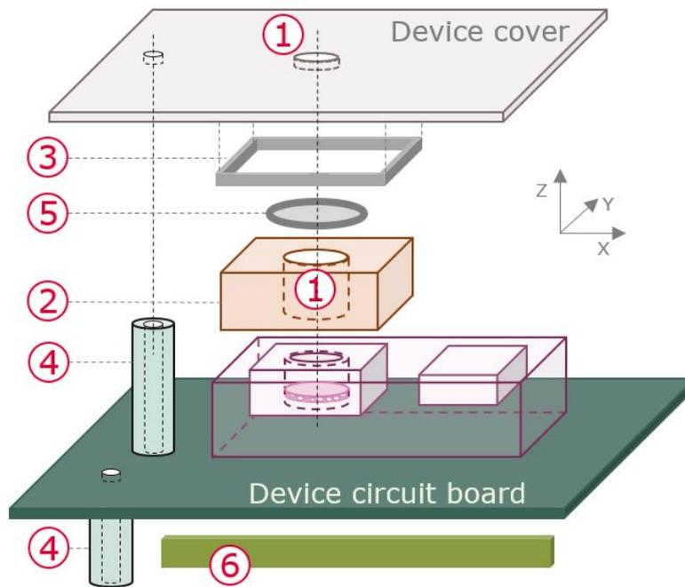
**Figure 5 MEMS microphone mechanical design**
