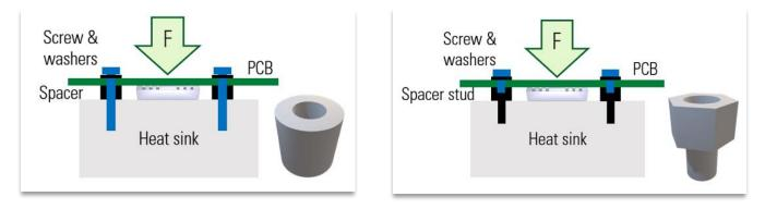
Figure 10. Mounting the SMPD using Cylindrical Spacers or Screw-type Spacer Studs
