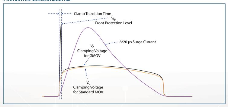
The Bourns® GMOV™ component protection characteristics are defined by Front Level Protection ( $V_{fp}$ ) and Clamping Voltage Level ( $V_c$ ).  $V_{fp}$  is measured with 10 % of peak current in accordance with IEC 61051-1. It should be noted that  $V_{fp}$  is a very short duration event, lasting less than 0.3  $\mu$ s.
