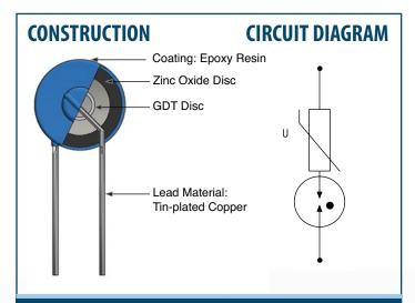
A GMOV<sup>™</sup> component functions when the GDT isolates the MOV from the circuit until such time as the voltage exceeds the turn-on voltage of the GDT. This isolation prevents the MOV from being damaged and prematurely failing from temporary overvoltage conditions below the turn-on voltage of the GDT.
