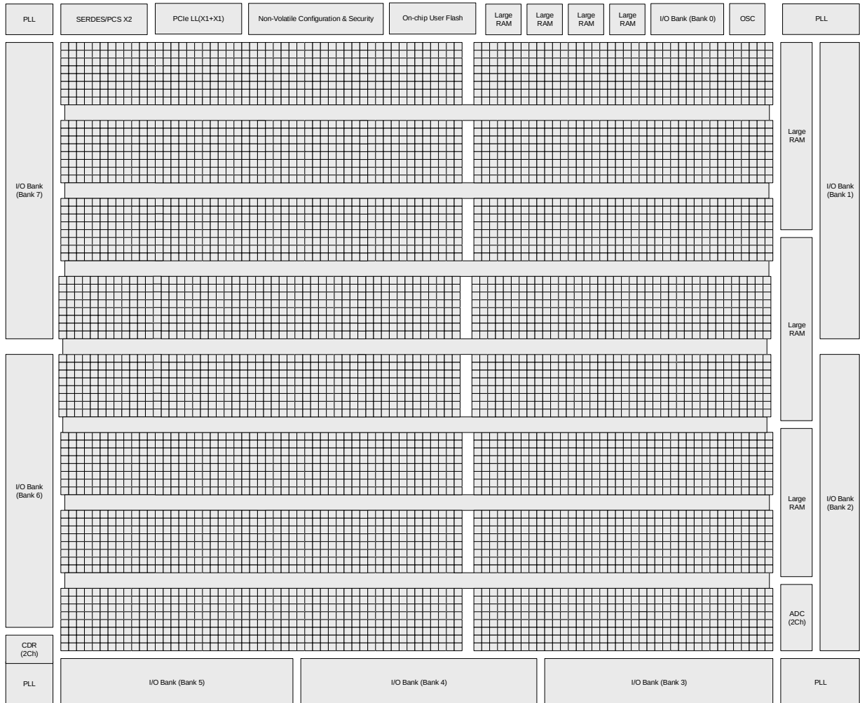
Figure 2.2. Simplified Block Diagram, MachXO5-NX-55T Device (Top Level)
