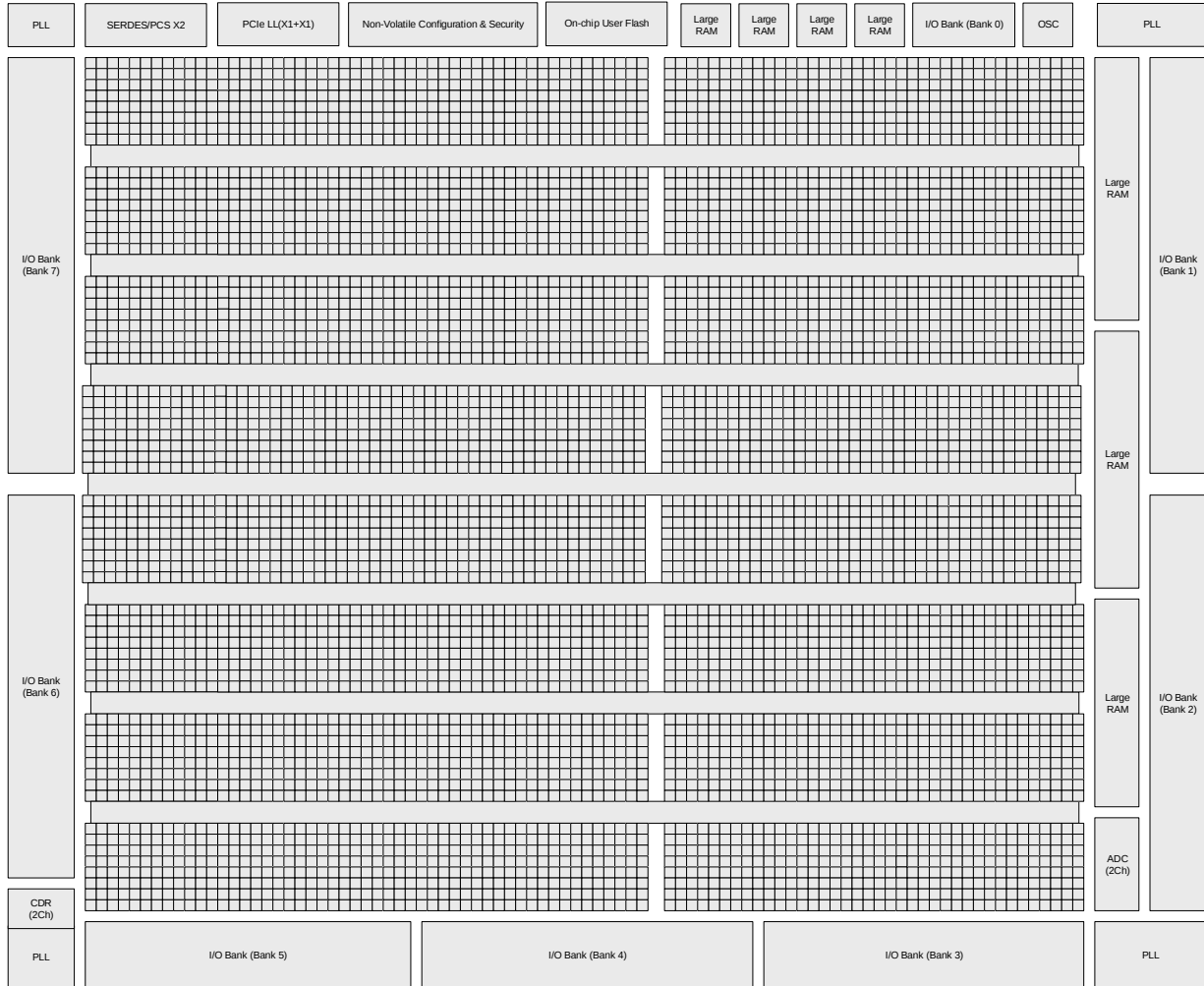
Figure 2.3. Simplified Block Diagram, MachXO5-NX-100T Device (Top Level)
