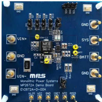
Figure 2: EV2672A-D-00A Evaluation Board
