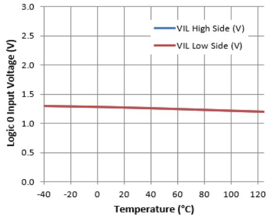
**Figure 23.** Logic 0 Input Voltage vs. Temperature
