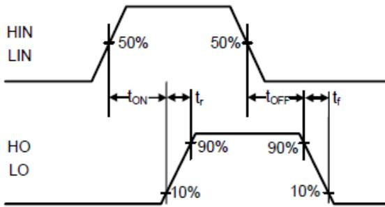
**Figure 1. Switching Time Waveform Definitions**
