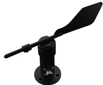
the RS485 wind direction transmitter utilizes a low-inertia wind vane to sense the wind direction. When the wind direction changes, the tail wing rotates to drive the axle magnet to rotate through the shaft, thereby obtaining accurate wind direction information. This transmitter can detect the 16 azimuths' natural wind directions. Typical applications include meteorology, ocean, environment, airports, ports, laboratories, industry, agriculture, and transportation.
