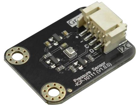
This sensor module also features a built-in temperature sensor for air pressure compensation and offers a temperature coefficient offset of  $\pm 0.5\text{ Pa}/^\circ\text{C}$ . Typical applications include UAV height control, indoor navigation and positioning, and vertical speed measurement.
