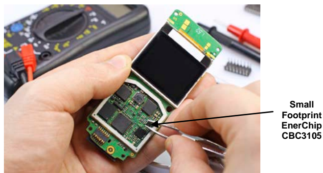
Figure 3: EnerChip CBC3105 used in a Mobile Phone Secondary Battery Application
