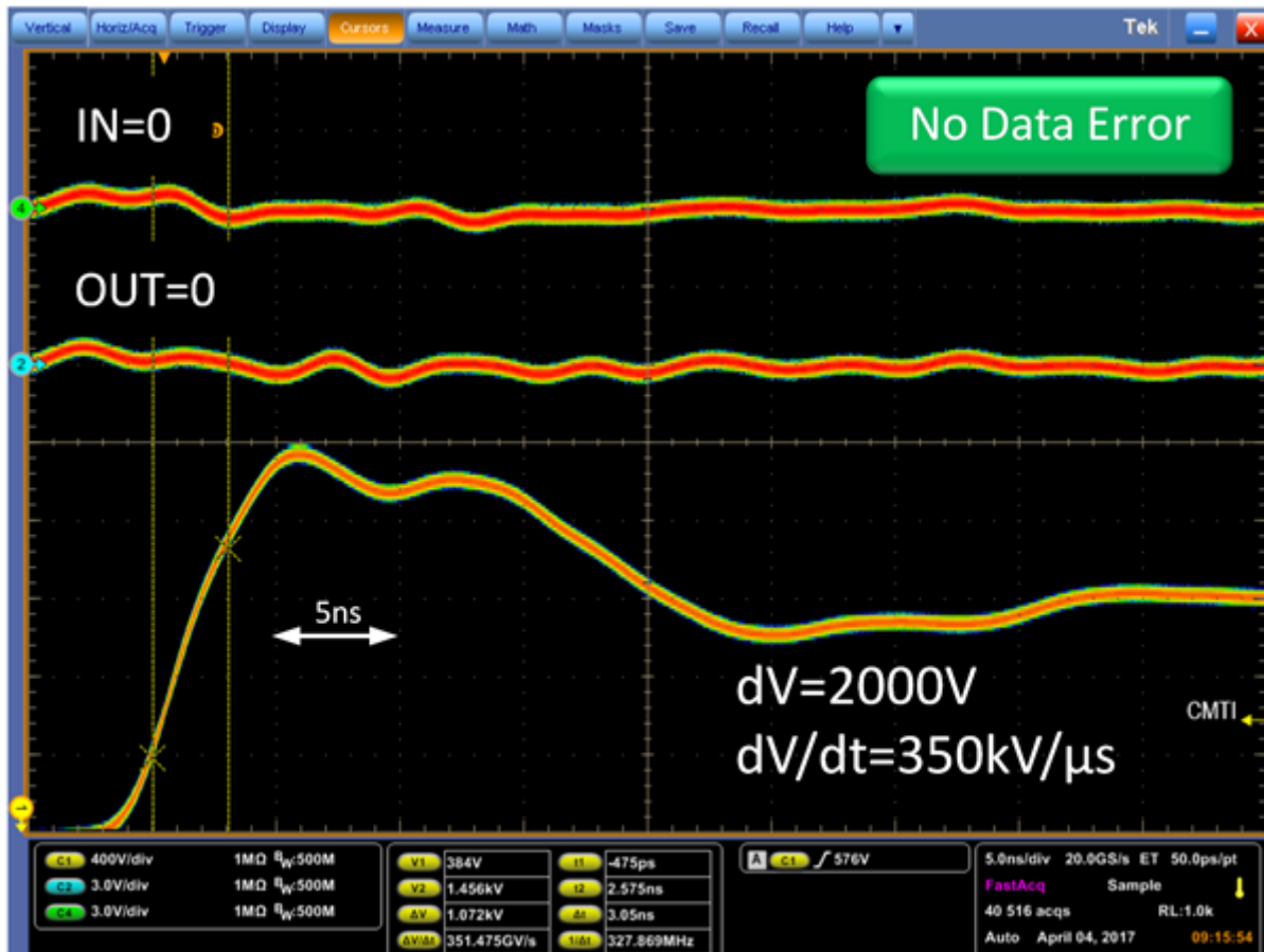
Figure 6. CMTI measurement of MAX22700.
