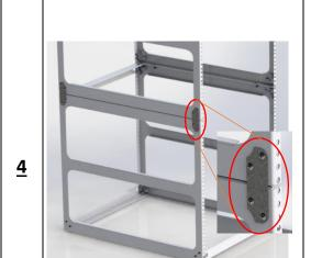
If using the rack in the horizontal position (17.5"/ 10 U) add mounting brackets **44-LMB-BT** on the outside of the side panels near every corner where 2 side panels rest on top of each other (see photo left). If using the rack in the vertical position (21.0"/12 U) add the shorter mounting brackets **44-SMB-BT**. See step 5 for final install information
