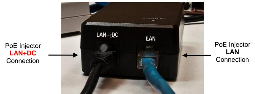
FIGURE 4 - PoE Injector's RJ45 Connections
