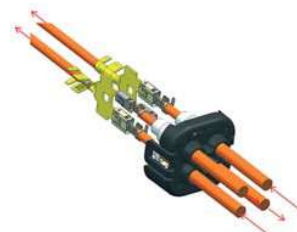
Terminal crimp wings are shown un-crimped.
