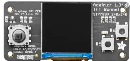
The 1.3" Color TFT Bonnet for Raspberry Pi features a Qwiic/STEMMA QT connector for I2C sensors and devices on the bottom. A kernel driver and Python library are available for the ST7789 chipset for using the TFT display. This 1.3" Color TFT Bonnet works with any Raspberry Pi computer, including the original Pi 1, B+, Pi 2, Pi 3, Pi 4, and Pi Zero.
