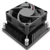
ATS fanSINKS™ feature cross-cut, straight aluminum fins. They support omnidirectional airflow for optimum cooling performance from attached fans and ambient air. The sinks are provided with a pre-assembled thermal interface material (TIM) to optimize heat transfer.
