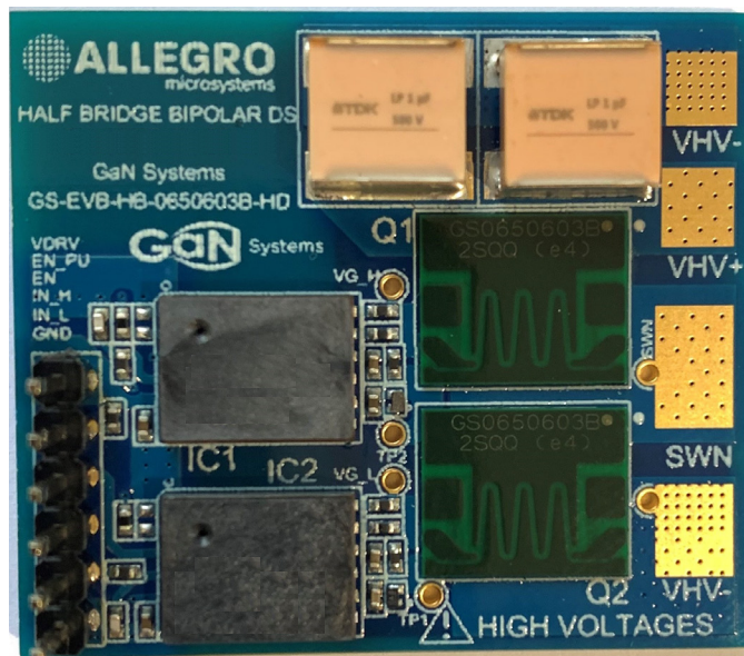
Figure 1: APEK85110 Demonstration Board
