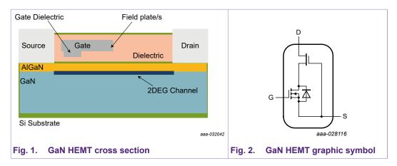
Fig. 2 shows how combining a low-voltage (LV; 30 V) robust Si MOSFET with the cascode configuration can eliminate all of the major concerns regarding the poor gate structures of the E-mode devices and make the entire usage very simple. An LV Si-based gate structure is a very mature technology and engineers are accustomed to using them.
