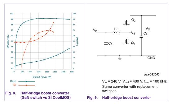
GaN FET losses are significantly lower due to the absence of reverse recovery losses and switching crossover losses. It is possible to achieve near ideal turn on and off losses with dV/dt of approximately 200 V/ns.
